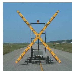
OPTION 2: L-893 LIGHTED RUNWAY CLOSURE MARKER
