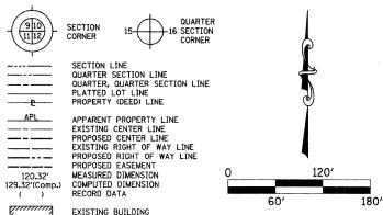
Bearings are referenced to the Illinois State Piane Coordinate System, East Zone, NAD 1983.
