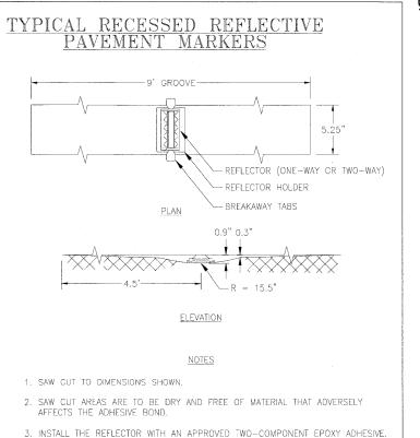
EPOXY SHOULD NOT OBSUCURE OR BLOCK THE LENS.
