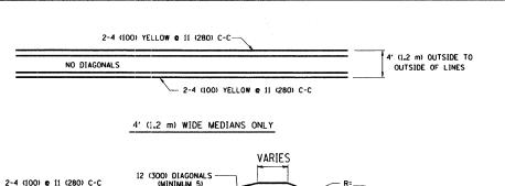
12 (300) DIAGONALS -(MINIMUM 5) FOR MEDIAN LENGTHS WHERE DIAGONAL SPACING CANNOT BE ATTAINED, USE 5 (FIVE) EQUALLY SPACED
