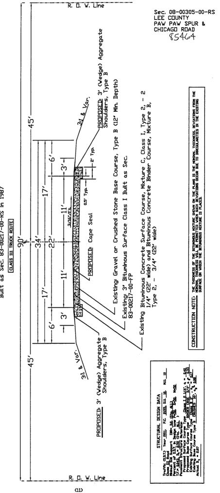
TYPICAL SECTION Chicago Road Sta, 54+61 to Sta, 108+43 (STATION EQUATION Sta, 57+02 Back = Sta, 7+00 Ahead) Built as Sec. 83-00217-00-RS in 1987
