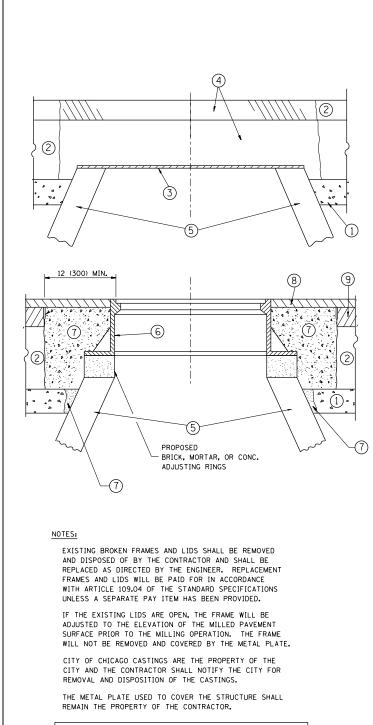
WHEN STRUCTURES ARE TO BE ADJUSTED OR RECONSTRUCTED, THE LOWERING AND RAISING OF THE FRAMES AND LIDS WILL NOT BE PAID FOR SEPARATELY BUT WILL BE INCLUDED IN THE COST OF THE CORRESPONDING PAY ITEM.
