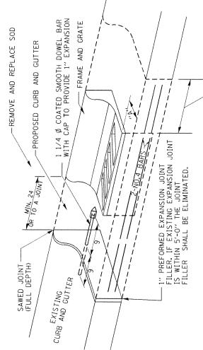
WHEN "A" IS GREATER THAN 2 , 2-NO. 4 BARS SHALL BE PLACED AS SHOWN.
