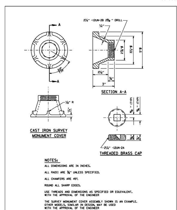
THE THREADS OF THE CAP AND COVER WILL BE COATED WITH PIPE TAPE OR PIPE THREAD COMPOUND PRIOR TO INSTALLATION.
