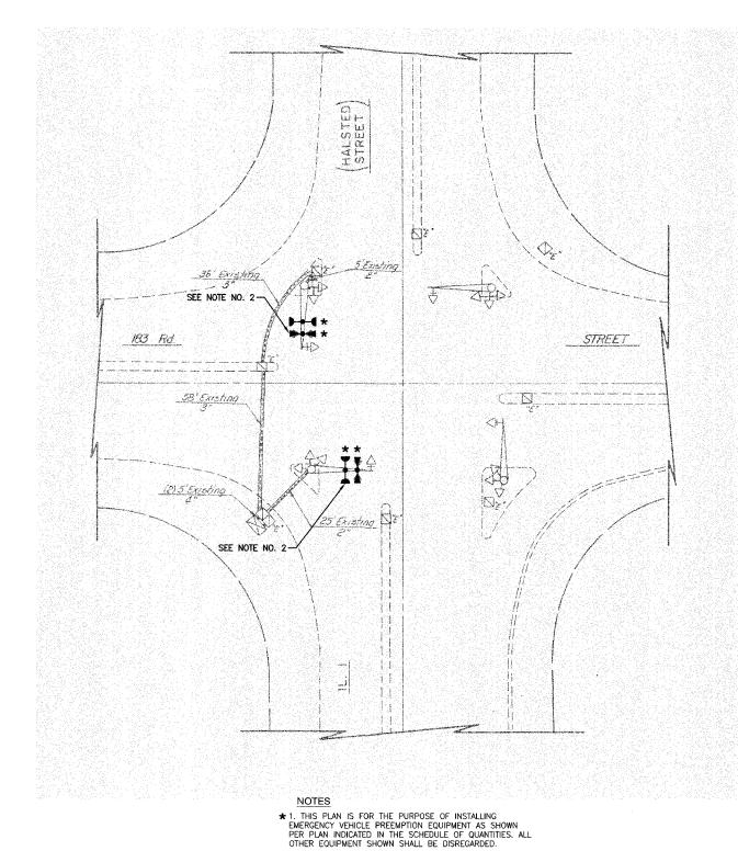
2. THE EXISTING EMERGENCY VEHICLE LIGHT DETECTOR AND LIGHT DETECTOR AMPLIFER SHALL BE REMOVED AND REPLACED WITH NEW EQUIPMENT. THE EXISTING EQUIPMENT SHALL BE RETURNED TO THE VILLAGE OF HOMEWOOD.
