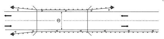
Bidirectional silver/silver should be used in lieu of monodirectional silver on both sides of two-lane bridges where the bridge pavement is less than 24 (610) wider than the pavement approaching the bridge.
