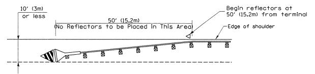
Traffic Barrier Terminal Type 1(Specia) [Terminal 10' (3m) or less from edge of shoulder]
