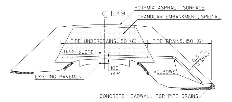
\*PIPE ELBOWS INCLUDED IN THE COST OF PIPE DRAIN ITEMS
