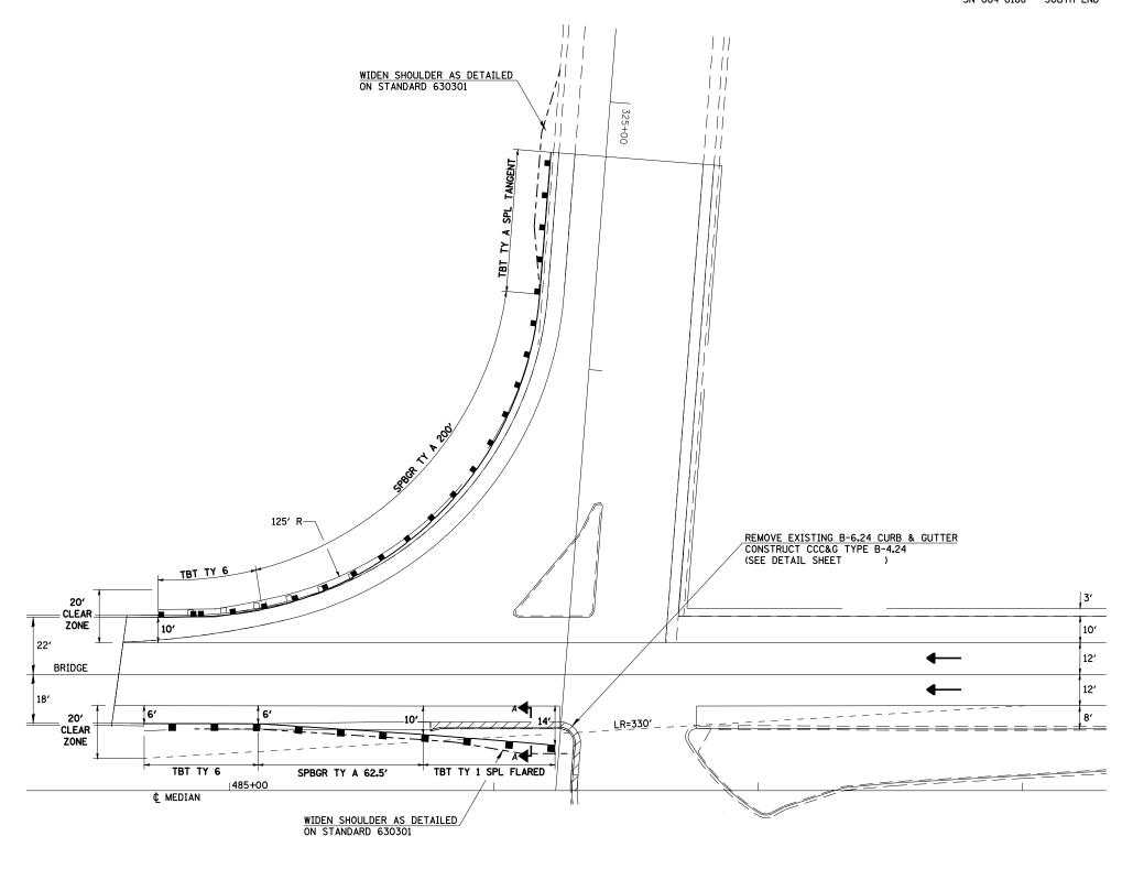
RAIL ELEMENTS FOR THE PROPOSED TRAFFIC BARRIER TERMINAL TYPE 6 AND STEEL PLATE BEAM GUARDRAIL TYPE A SHALL BE FABRICATED WITH A 125' RADIUS
