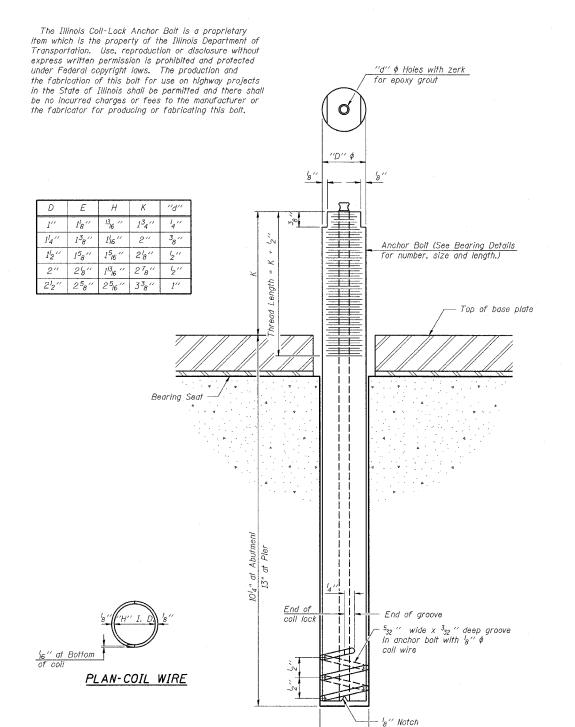
ILLINOIS COIL-LOCK ANCHOR BOLT
