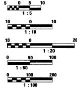
FULL SIZE PLANS HAVE BEEN PREPARED USING STANDARD ENGINEERING SCALES, REDUCED SIZED PLANS WILL NOT CONFORM TO STANDARD SCALES, IN MAKING MEASUREMENTS ON REDUCED PLANS, THE ABOVE SCALES MAY BE USED.
