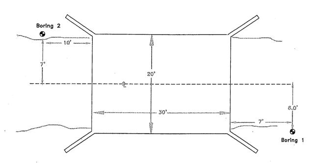
Note: Center of Existing Bridge Deck Assumed Benchmark Elevation = 100.0. 403.21
