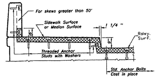
**CONTINUOUS SEAL TYPE NEOPRENE EXPANSION JOINTS**
