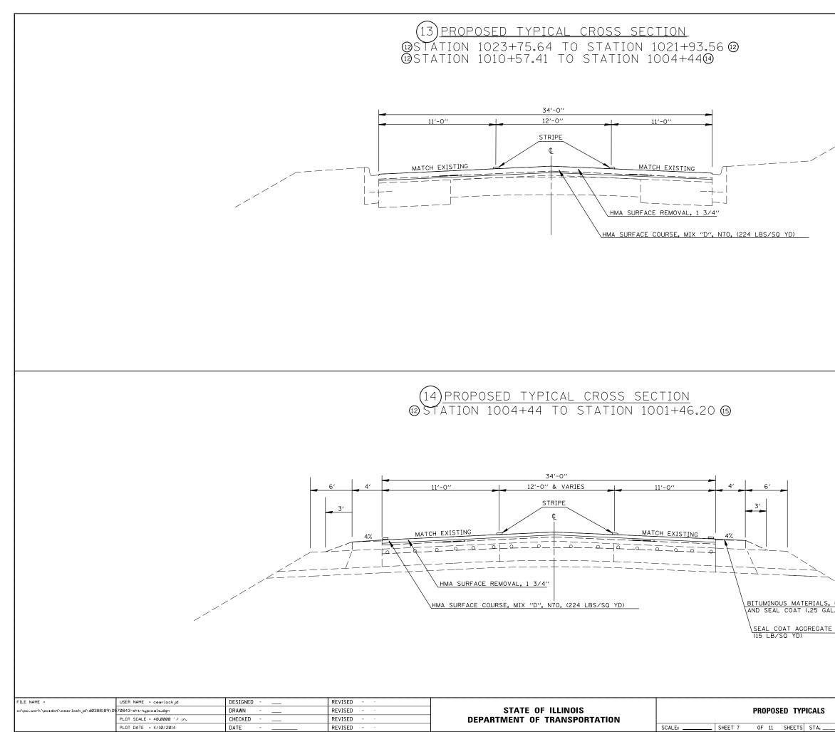
BITUMINOUS MATERIALS, COVER (AND SEAL COAT (.25 GAL./SQ YD)
