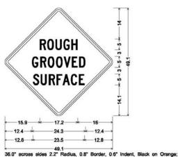
36.0" across sides 2.2" Radius, 0.8" Border, 0.6" Indent, Black on Orange [ROUGH] C 2K 81% spacing; [GROOVED] C 2K 91% spacing; [SURFACE] C 2K 85% spacing;
