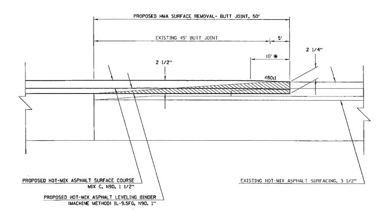
\* TAPER HMA LEVELING BINDER FROM 3/4" TO 1" IN 10'
