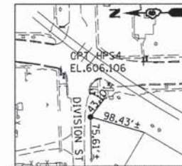
CONTROL POINT #HPS4 SET I.P. 7' SOUTH OF SOUTH EDGE OF DIVISION STREET AND 42' WEST OF RAILROAD SIGNAL IN SW QUADRANT N 1,146,493.2417 E 2,444,269.0733 ELEV. 606.106
