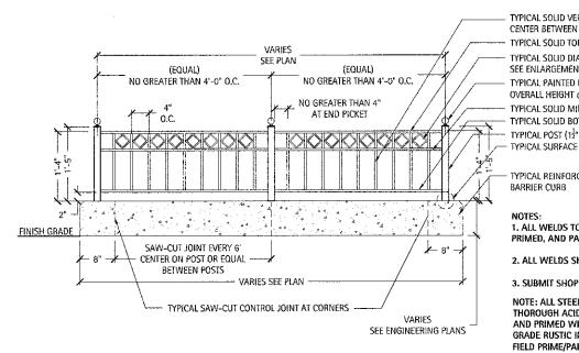
TYPICAL SOLID VERTICAL PICKET (1/2" SQ. – STEEL TUBE) – 4" O.C. CENTER BETWEEN POSTS
