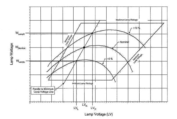
Ballast Regulation =  $\frac{W_{LampH} - W_{LampL}}{W_{LampN}} \times 100$
