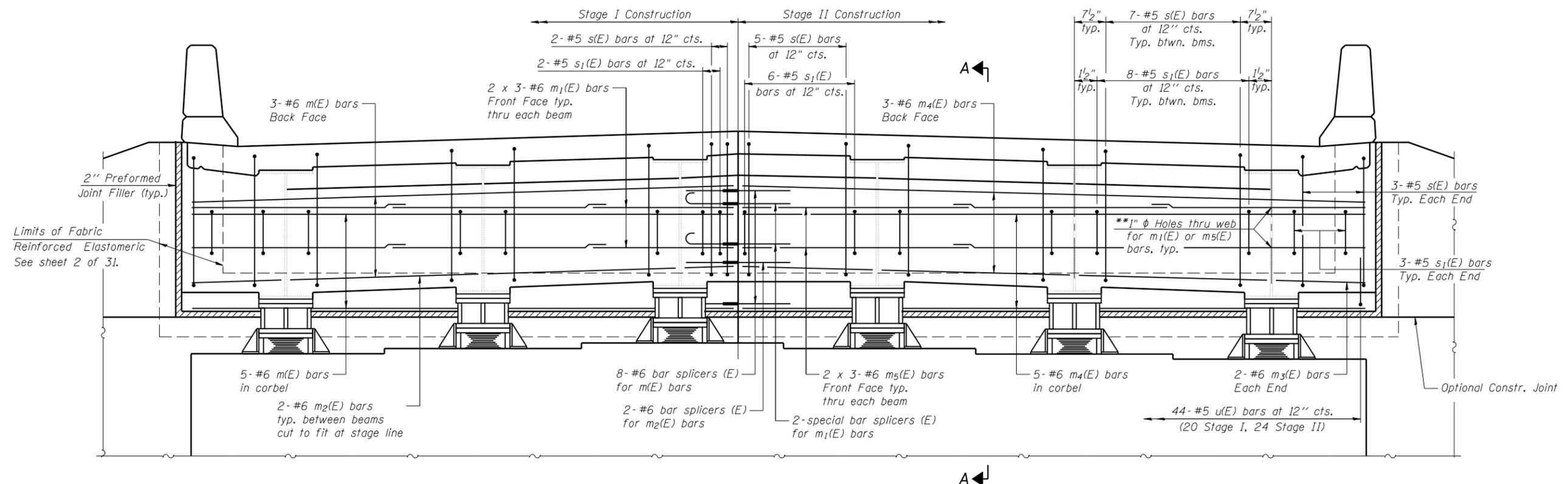
**DIAPHRAGM ELEVATION AT ABUTMENT**
