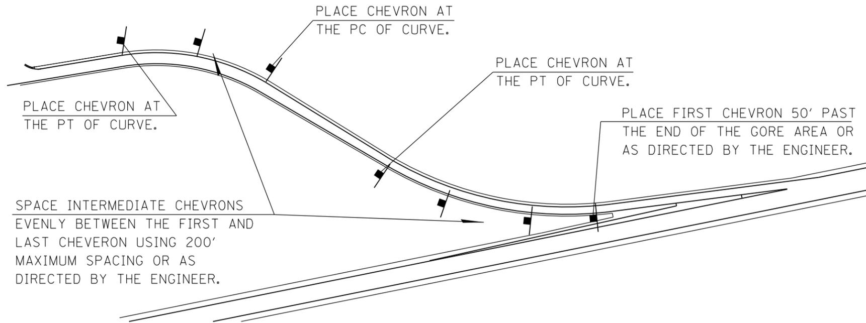
SPACE INTERMEDIATE CHEVRONS EVENLY BETWEEN THE FIRST AND LAST CHEVRON USING 200' MAXIMUM SPACING OR AS DIRECTED BY THE ENGINEER.
