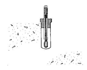
5. The exact method for <u>surface</u> and <u>sub-surface</u> concrete temperature monitoring shall be indicated in the contractor's cold weather concreting plan. The maximum permissible difference between the interior and surface temperature is 35 °F. Adjustments in protection method shall be implemented if the maximum permissible difference is exceeded.
