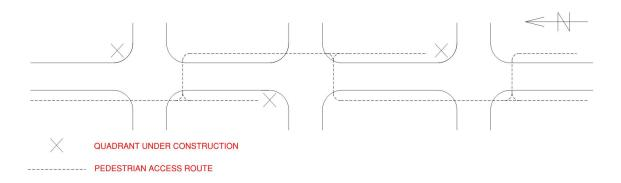
Only one quadrant per block is under construction. This allows access to every building on the main route and an uninterrupted pedestrian access route.
