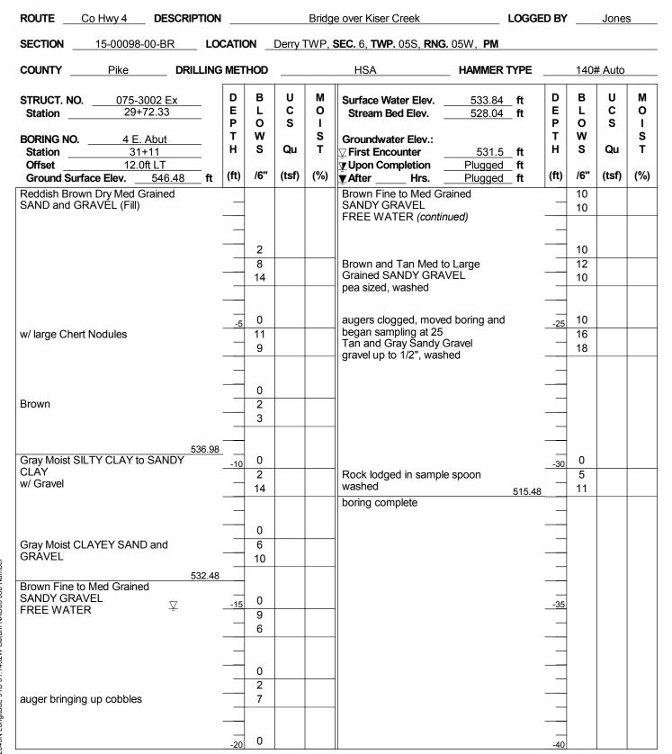
The Unconfined Compressive Strength (UCS) Failure Mode is indicated by (B-Bulge, S-Shear, P-Penetrometer, E-Estimated) Abbreviations W.O.H - Sampler Advanced By Weight of Hammer, W.O.P - Advanced by Weight of Pipe, B.S. - Before Seating The SPT (N value) is the sum of the last two blow values in each sampling zone (AASHTO T206) BBS, from 137 (Rev. 8-99)
