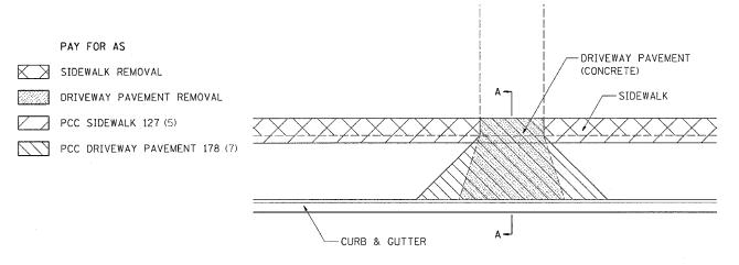
1.5m (5') -178mm (7") CONSTRUCTION OR SAWED JOINT DRIVEWAY PAVEMENT -DEPRESSED SECTION A-A CURB & GUTTER
