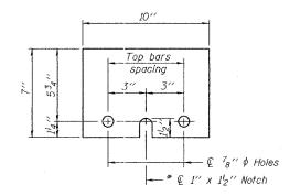
STEEL RETAINER P I" x 7" x 10" \* Required only with Detail II
