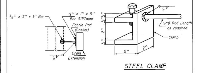
Notes: Pop rivet the 'B'' x 1'' bar to Drain Extension. Weld or securely attach rod to both the clamp and bar stiffener.
