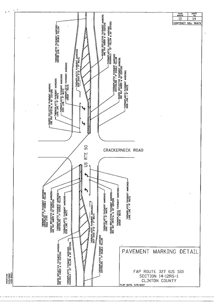
TOTAL SHEETS CONTRACT NO.: 76A79 THERMOPLASTIC PAVEMENT MARKINGS-EDGE LINE - 4" WHITE SHOULDER 20,-0,, CHEWAY CRYSTAL & 40' CENTERS SHOUL DER SHOULDER RAISED REFLECTIVE PAVEMENT MARKER. ONEWAY CRYSTAL B 40' CENTERS HIGHWAY 50 THERMOPLASTIC PAVEMENT MARKINGS -EDGE LINE - 8" WHITE GORE MARKING SHOULDER LIMITS OF RESURFACING-AT RAMPS SHOULDER TYPICAL RAMP DETAIL FAP ROUTE 327 (US 50) SECTION 14-12RS-1 CLINTON COUNTY PLOT DATE: 3/21/2007
