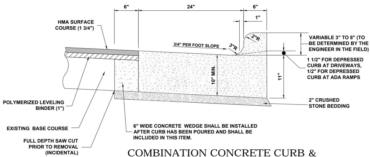
**COMBINATION CONCRETE CURB & GUTTER TYPE B-6.24 (MODIFIED)**
