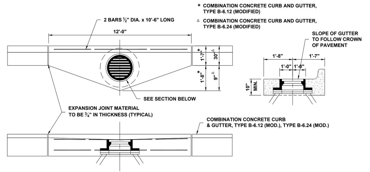
**GUTTER AT DRAINAGE STRUCTURE**
