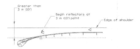
NOTE: Omit terminal marker when terminal over 3 m (10') from edge of paved shoulder or break point of unpaved shoulder, or when terminal buried in backslope.
