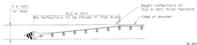
Traffic Barrier Terminal Type 1(Specia) [Terminal 3 m (10') or less from edge of shoulder] All dimensions are in millimeters (inches) unless otherwise noted.
