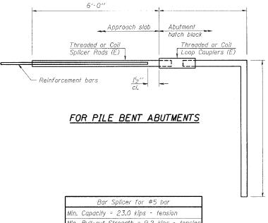
Min. Pull-out Strength = 9.2 kips - tension No. Required =
