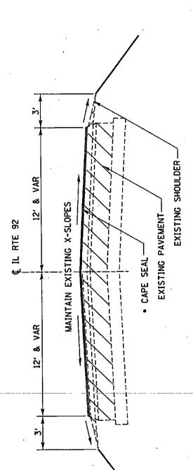
• CA 16, FAI SPECIAL AGGREGATE GRADATION FOR A-1 SURFACE TREATMENT MICRO-SURFACING, SINGLE PASS, TYPE II, 13 KG/SO M (24 LB/SO YD)" TYPICAL SECTIONS
