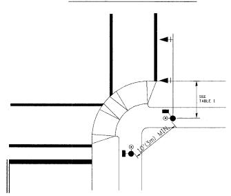
RECOMMENDED PUSHBUTTON LOCATIONS FOR ACCESSIBLE PEDESTRIAN SIGNALS SHALL BE IN ACCORDANCE WITH THE CURRENT MUTCO (SEE NOTE 1). TO MEET MUTCD REQUIREMENTS, PEDESTRIAN SIGNAL PUSHBUTTONS MAY HAVE TO BE MOUNTED ON A SEPARATE POST.
