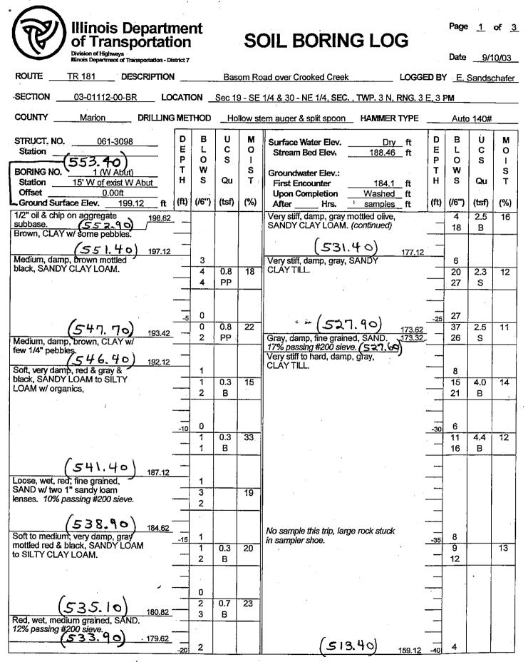
The Unconfined Compressive Strength (UCS) Failure Mode is indicated by (B-Bulge, S-Shear, P-Penetrometer) The SPT (N value) is the sum of the last two blow values in each sampling zone (AASHTO T206)
