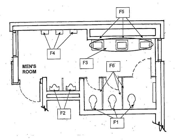
F1 - FIXTURE : WATER CLOSET HARDWIRED FLUSH VALVE
