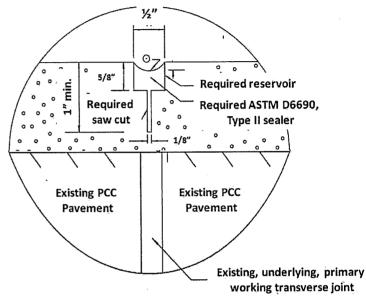
Methods not shown herein for equipment used to obtain the sawed joint detailed may be proposed by the Contractor to the Department at the pre-construction meeting. The proposal shall include a complete list of equipment to be used and locations where equipment has previously been used with success.
