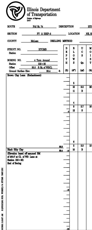
An assumed centerline elevation of 100.00 and station of 10+00 is used when this in The Unconfined Compressive Strength (UCS) Failure Mode is indicated by (B-Bulge, j The SPT (N Value) is the sum of the last two blow values in each sampling zone
