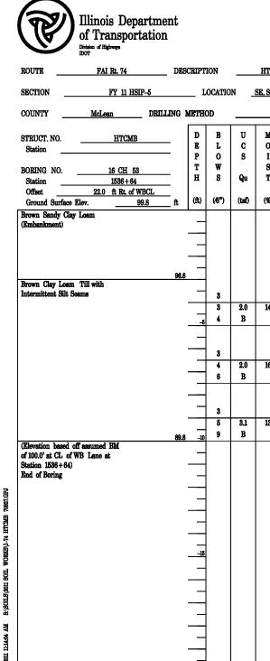
An assumed centerline elevation of 100.00 and station of 10+00 is used when this i The Unconfined Compressive Strength (UCS) Failure Mode is indicated by (B-Bulge, The SPT (N Value) is the sum of the last two blow values in each sampling zone
