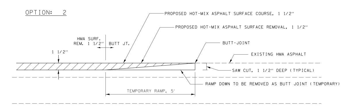
NOTE: RAMPING DOWN DURING HOT-MIX ASPHALT SURFACE REMOVAL, 1.5" WILL NOT BE PAID FOR AS TEMPORARY RAMP.
