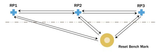
Figure 5. Three reference points tie to new reset bench mark.
