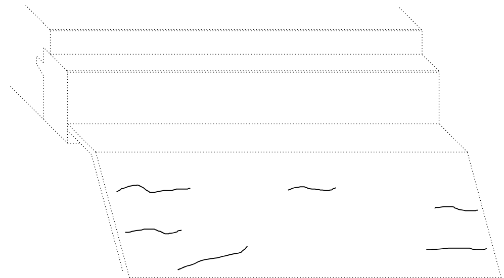
SOUTH SLOPE WALL Approximately 40 linear feet of crack to seal
