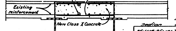
RECONSTRUCTED LONGITUDINAL JT.
