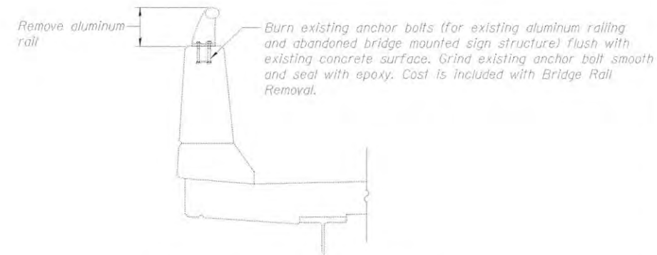
REMOVAL DETAILS SECTION EXISTING SOUTH PARAPET
