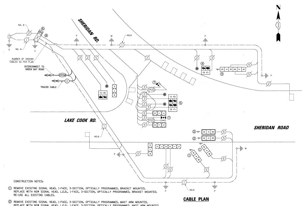
REPLACE WITH NEW SIGNAL HEAD, L.E.D., 1-FACE, 3-SECTION, OPTICALLY PROGRAMMED, MAST ARM MOUNTED. RE-USE ALL EXISTING CABLES.
