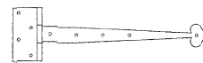
GATE HINGE DETAIL NOT TO SCALE ACORN MANUFACTURING 9" HEART SHAPE STRAP HINGE, SIGNATURE HARDWARE OR APPROVED EQUAL
