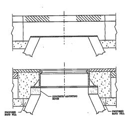
DETAILS FOR FRAMES AND LIDS ADJUSTMENT WITH MILLING
