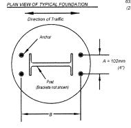
B (Bracket No. 1) = Depth of Post + 202mm (7-15/16") B (Bracket No. 2) = Depth of Post + 205mm (8-1/16")
